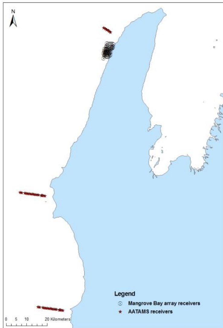
Fig. 1. Ningaloo showing the approximate location and length of the receiver curtains and the receiver array in the northern part of the region at Tantabiddi. Because the shelf south of Point Cloates is much wider, the receiver curtain there must be approximately 22 km long to reach the 100 m depth contour.
