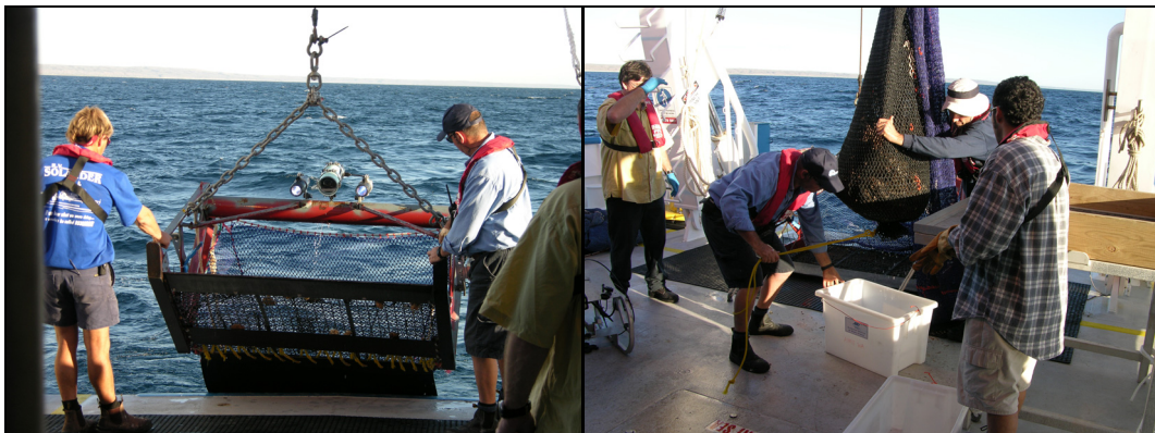
Figure 5.7: Epi-benthic sled sampling: Left – deployment of the epi-benthic sled showing the large opening of the sled and the location of the stills camera and associated lights. Right – the epi-benthic sled suspended by the capstan winch (out of frame) showing the cod end distended with sample material.
