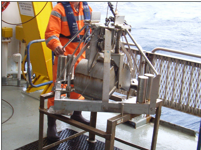
Figure 4.1: The Smith-McIntyre bottom sediment sampler that was operated from the starboard deck of RV Solander.
