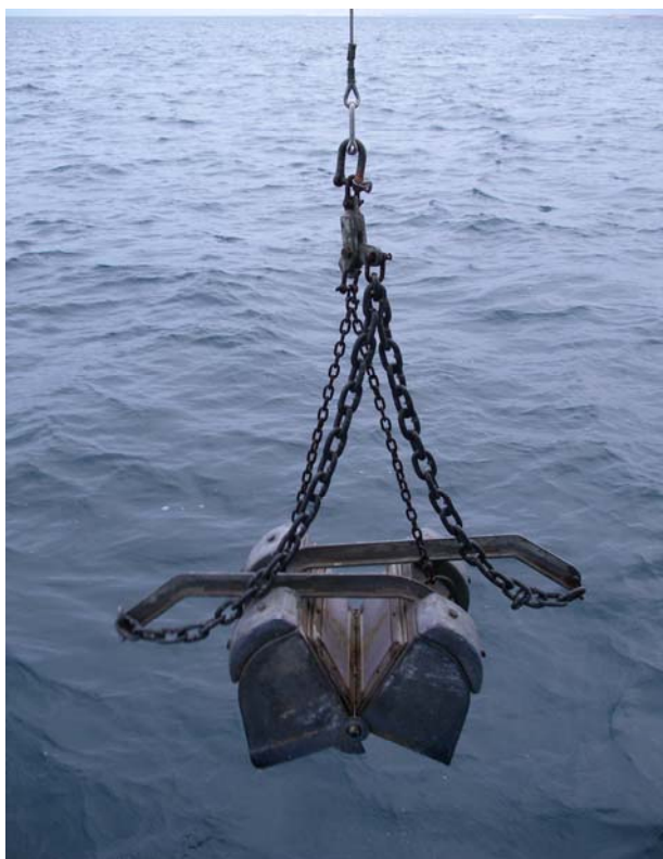
Figure 9. van Veen grab sampler for collecting surface and surface material to a depth of ~10 cm.
