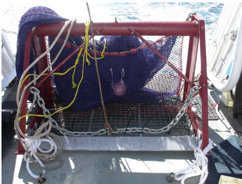
Figure 16. New benthic sled used to sample taxa from targeted communities in 2007.
