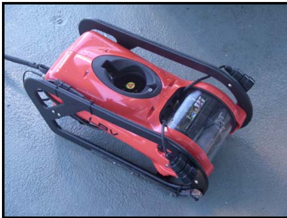
Figure 14 (a) LBV ROV Seabotix remote operated vehicle (b) ROV operating console
