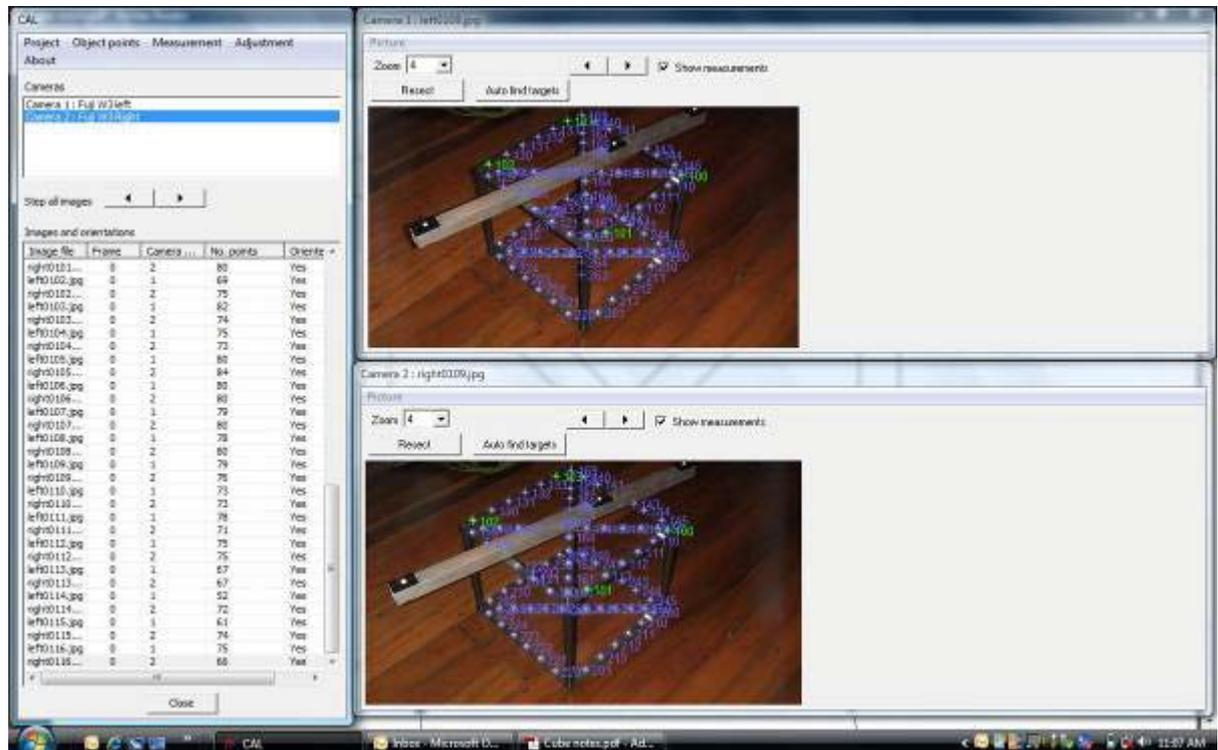
**Figure A 1:** Screen grab of CAL calibration process. Calibration was performed using 36 images of the calibration cube (1 stereo image set from 4 camera rotations, from 9 different views of the calibration cube). All images were captured at approximately 60cm from the calibration cube.
