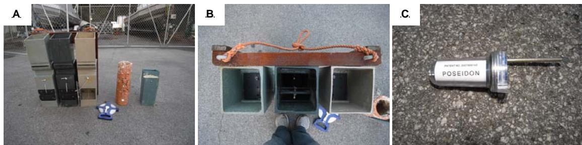
**Figure 12a-c:** Octopus trap types deployed during pilot study; a) LCD, cement and PVC trap designs, b) LCD trap configuration. Note the two traps outside have trap doors shut, the middle one has its LCD light flashing and c) the LCD light used in the trap which flashes every 5 secs.
