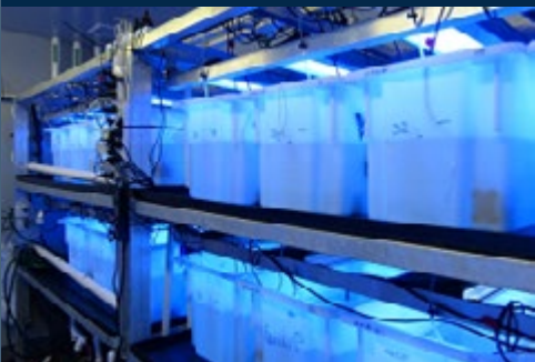
Figure 2 - Overview of part of the experimental set-up in the climate-controlled experimental room at the Australian Institute of Marine Science. Corals were maintained in aquaria with high water flow and aeration. Aquaria were placed inside plastic tanks to create a closed system and illuminated with actinic fluorescent lights.
