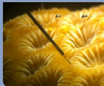
Figure 1. fiber-optic microsensor inserted into the coenosarc tissue of the examined coral species, measuring the amount of light available for photosynthesis within the coral tissue in increments (step sizes) of 100 \mu\text{m} .
