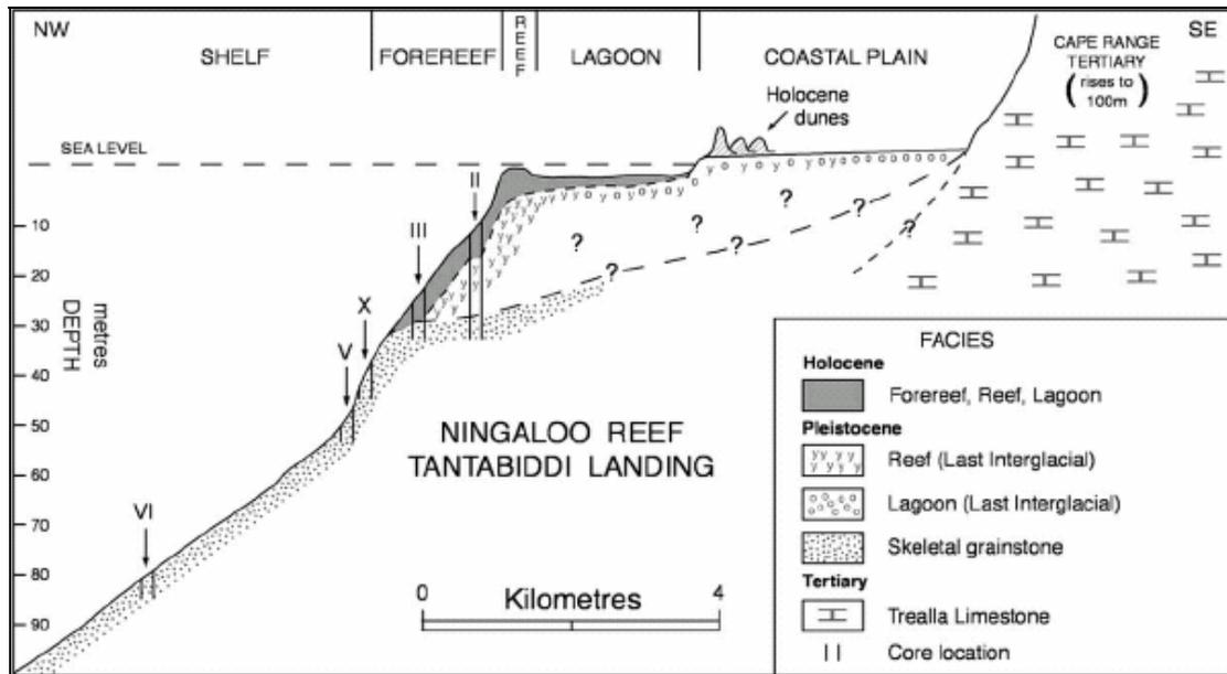
Figure 8. Idealised northwest-southeast cross section of northern Ningaloo Reef based on the cored transect and seismic data at Tantabiddi (Collins et al. 2003).
