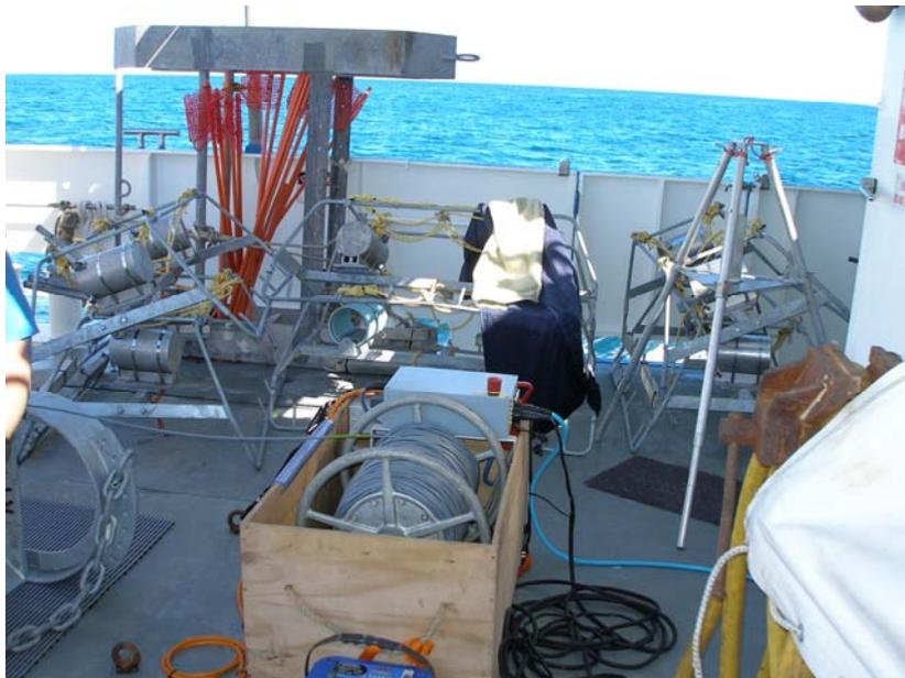
Figure 34. Towed video winch and electromechanical cable
