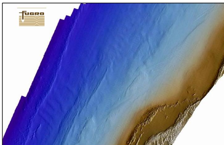
Figure 14. Multibeam bathymetry image of Osprey SZ showing ridge systems on the mid and outer shelf.
