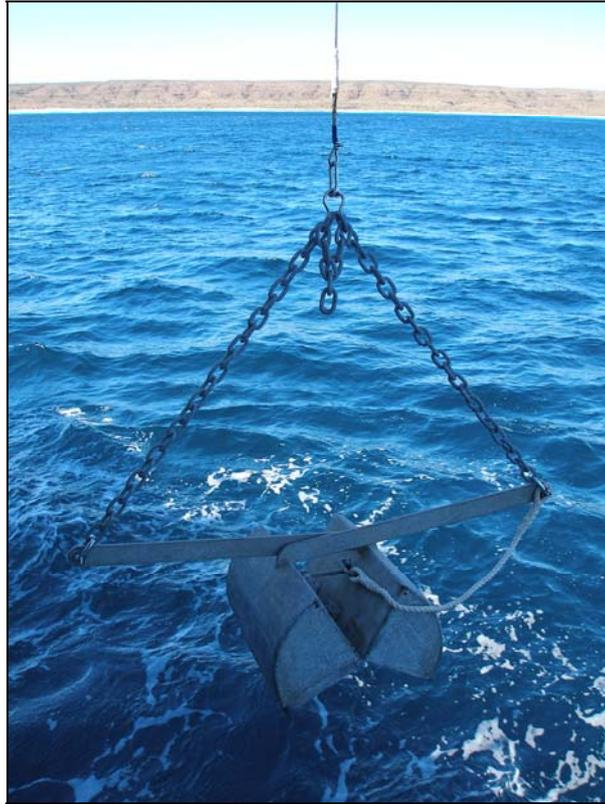
Figure 10. van Veen grab sampler for collecting surface and subsurface material to a depth of ~ 10 cm from the northern part of the NMP.
