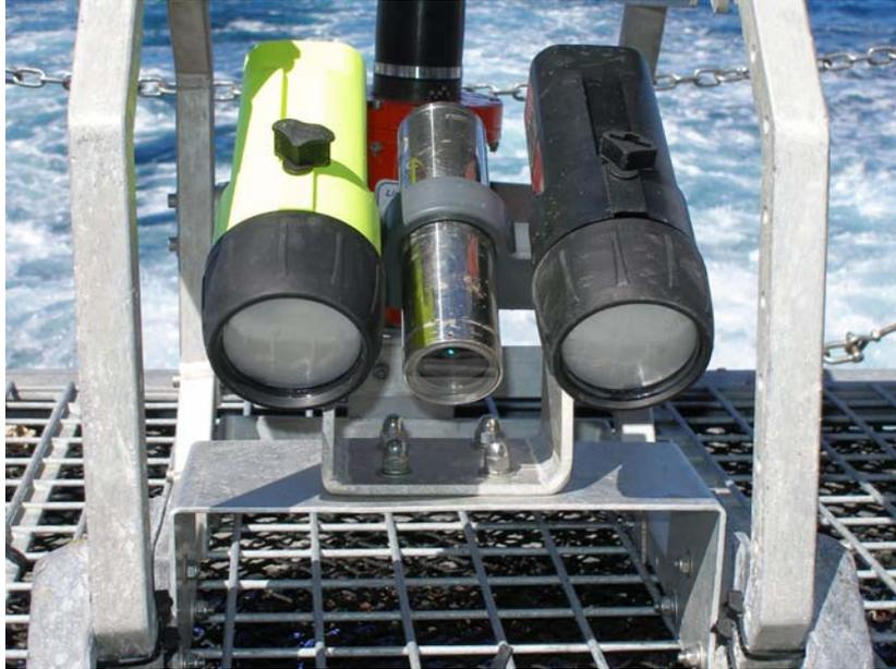
Figure 33. Towed video vane with video camera and lights
