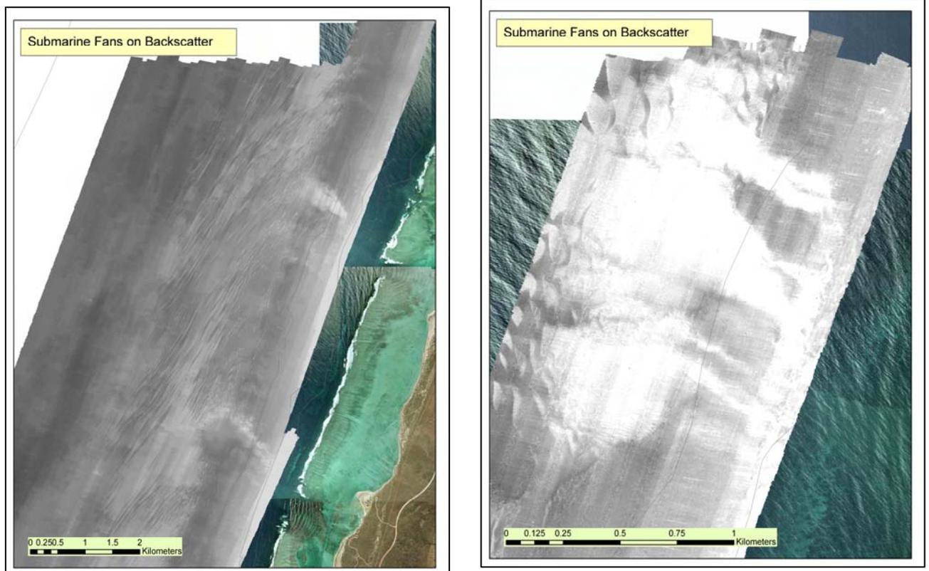
Figure 12. a) Backscatter image of submarine fan sediments b) Close up of fans and dunes
